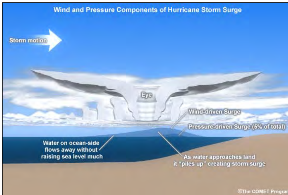
Figure 4.2 Wind and Pressure Components of Hurricane Storm Surge (Source: NHC)
